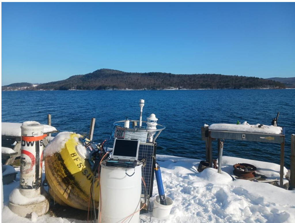
Testing the whole system with the new Airmar weather station. (Credit: Kiyoko Yokota)
