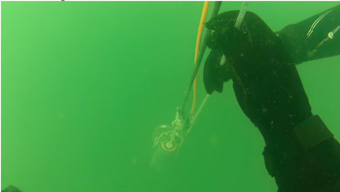
A Biological Field Station Volunteer Dive Team member, Alex Sessions, checking the data cable (black) and the thermistor array (orange cable) underwater. (Credit: Alex Sessions)
