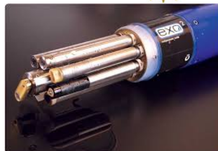
EXO 2 sonde with multiple probes for different water quality parameters
