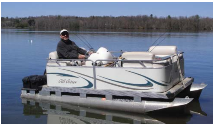
Bill Elsey in his 13’ electric pontoon boat GILL GETTER which can go 2 hrs. at 4mph or 10 hrs at 3mph; Photo by Tim Pokorny.
