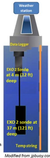
EXO 2 sonde with multiple probes for different water quality parameters
