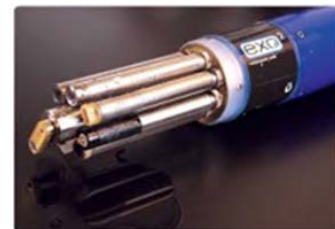
EXO 2 sonde with multiple probes for different water quality parameters
