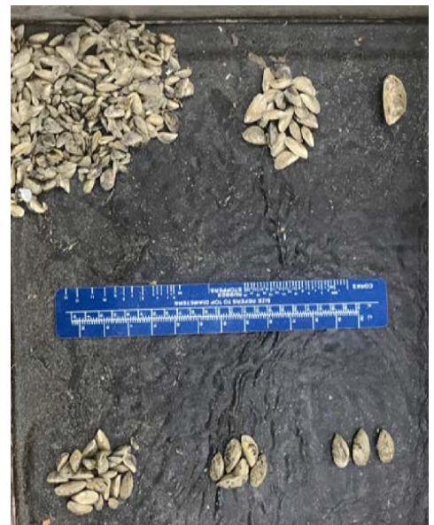
ABOVE: Sample of mussels from Village of Cooperstown water intake separated by apparent age classes. Quagga mussels at top; Zebra mussels at bottom; Photo by Paul H. Lord. BELOW: Pigging the Water Line; Photos by Peter Regan
