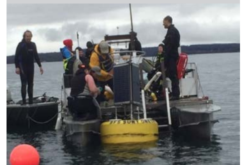
ABOVE AND BELOW: Final stage of the data buoy deployment occurring on the 90 HP jon boat - Anodontoides (large pontoon) complex. This year the upper portion of the buoy system, containing the weather station and solar panels, was secured on top of the lower portion at the deployment site rather than on shore. This reduced the risk of damage to the upper part in transit. Photos by Wayne Bunn
